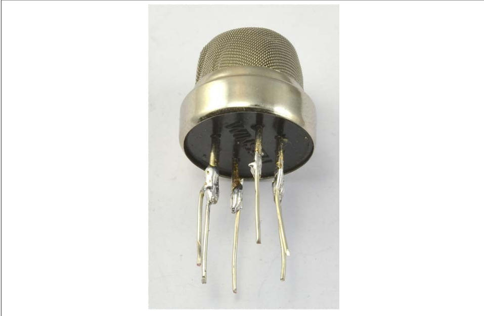
Figure 12-5. Soldering leads onto the gas sensor
